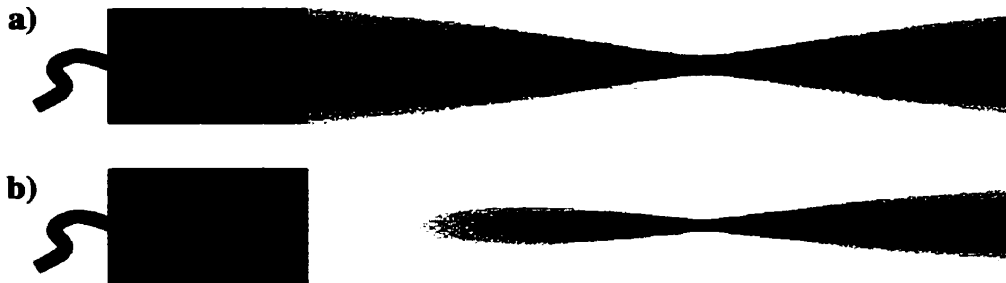
Figure 54: a) Sketch of the two-way sensitivity pattern for conventional imaging; b) sketch of the two-way sensitivity pattern for tissue harmonic imaging. Tissue harmonic imaging is insensitive to scattering from superficial layers.
