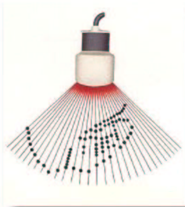
Figure 2.8: A linear array transducer can be used to create a B-Mode image [5].
