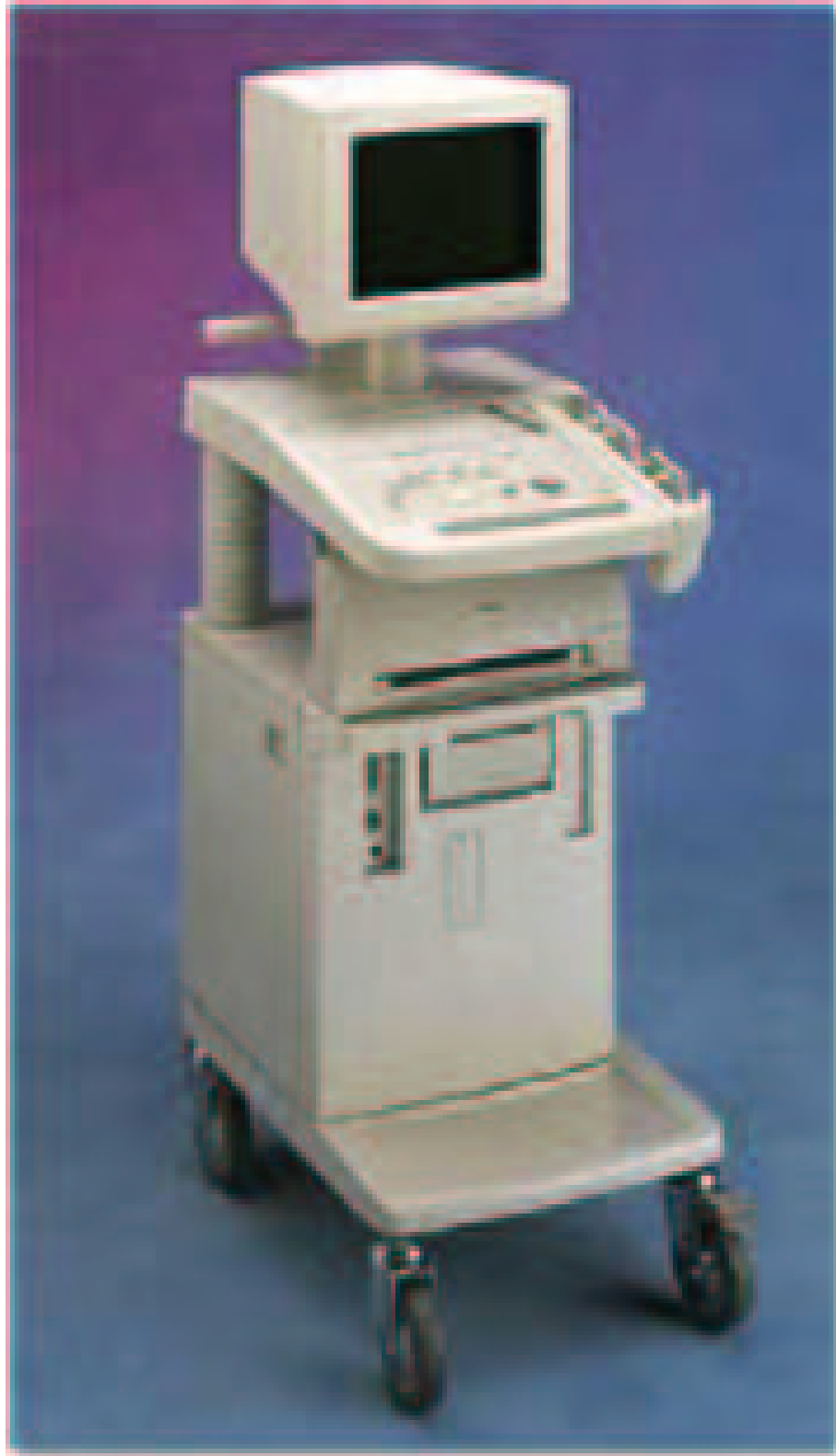
Figure 2.4: A typical medical ultrasound system. The display section is a CRT monitor [4].
