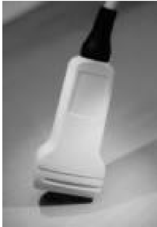
Figure 2.12: A typical linear array transducer [3].
